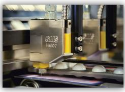
Works with almost any kind of hot melt, including fugitive, permanent, remoistenable or pressure sensitive adhesives
